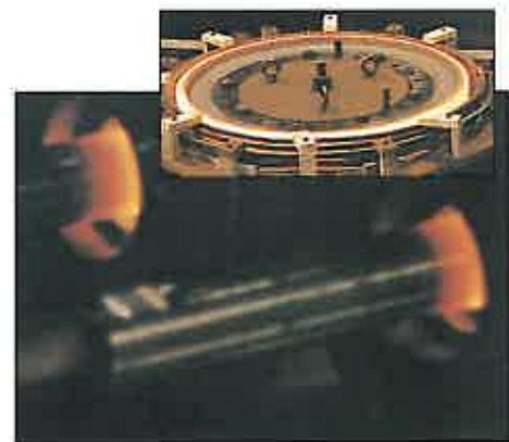
“Induction heat treating chain pins.”
